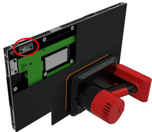
The special designed assembling adapter should be used when the panels are connected vertical. With the use of the adapter, it is ensured, that the panels are aligned correctly. Each device has four captive screws and four recessed magnets. The magnets atomically attach the adapter to the corners of the panel.
