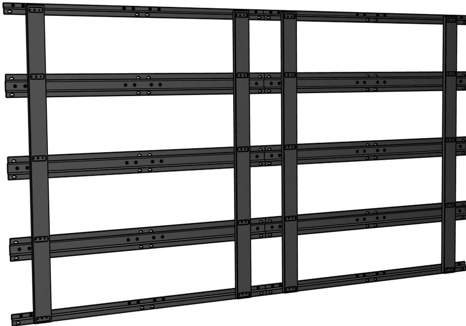
Prior to the wall mounting bas installation on the wall, we need to connect the wall mounting bars with the supplementary mounting bars. For an installation with 2x4 screens, two mounting bars and five wall mounting bass are necessary. A 4x4 screen installation is mounted with twice as much bars. Each wall mounting bas is attached to the mounting bar by four screws. The total installation depth of the screen will not exceed 37mm.
