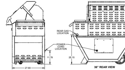
**GAS REQUIREMENTS:** 1/2" NPT gas connection. Minimum gas supply is 7" water column for natural gas and 11" for propane. Operating pressure at the manifold is 4" water column for natural gas and 10" for propane. All units require a regulated gas supply. (included)
