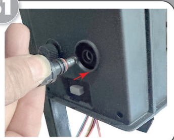
Plug the adapter into the corresponding hole of the control box. (See Figure 31)
