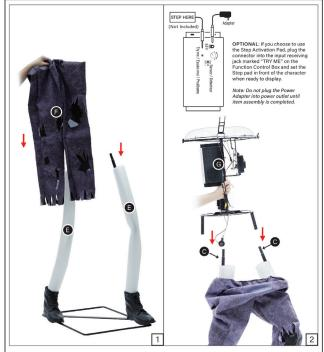
Slide the (F) Pants over the (E) Foam Tubes as shown in Figure 1. Attach the (G) Body Frame to the (C) Upper Support Poles as shown in Figure 2.
