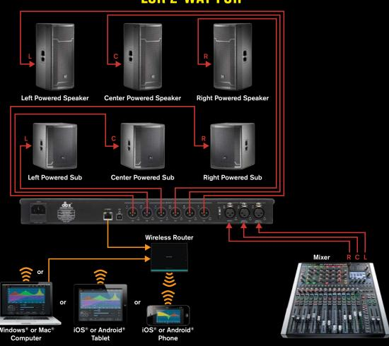
Analog Audio Connection Ethernet Connection Wi-Fi Signal Left Signal Center Signal Right Signal
