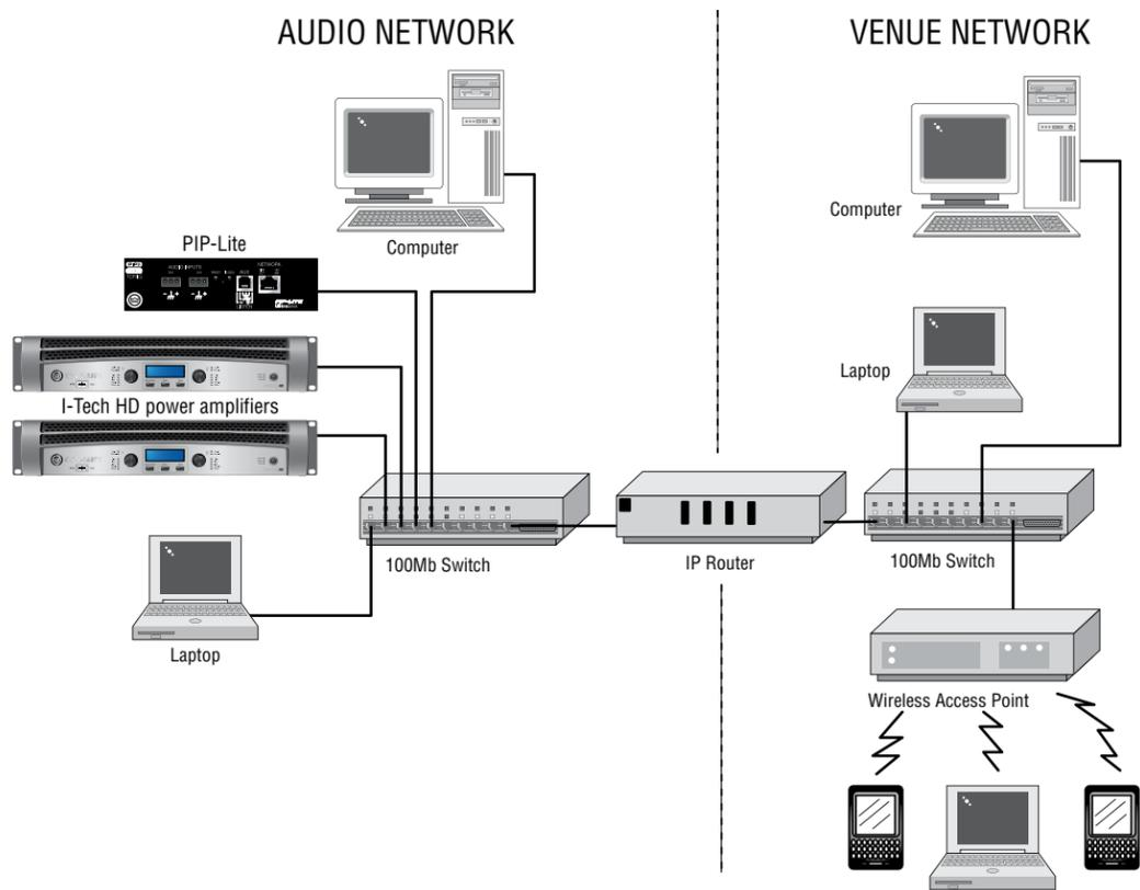
Figure 9.2 Multiple-Network Communication Via an IP Router
