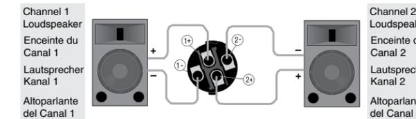
Figure 2.10 Wiring Two Stereo Speakers
