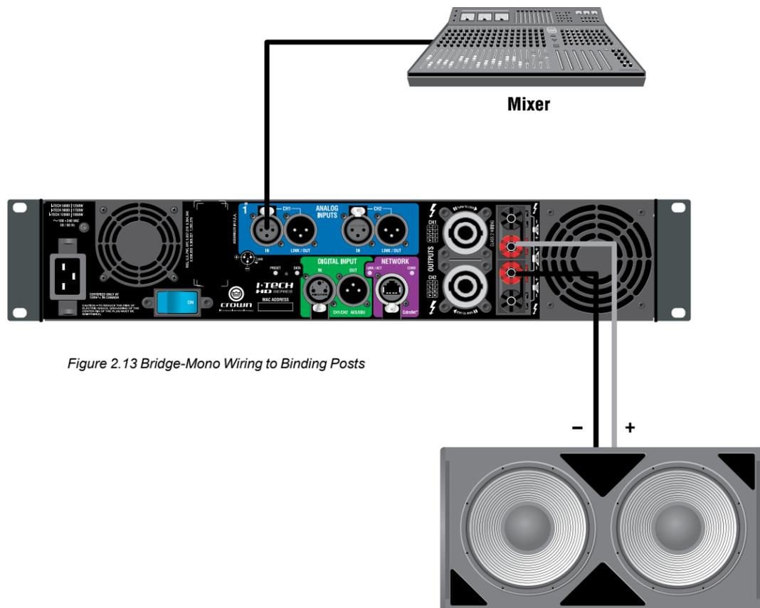
Figure 2.13 Bridge-Mono Wiring to Binding Posts
