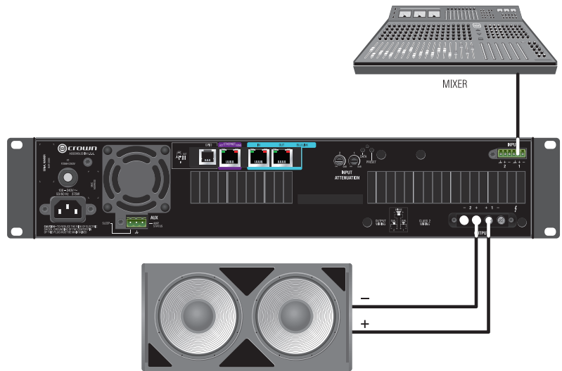
Figure 21 System Wiring Bridge Mode
