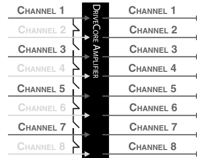
Figure 4.6.5 Four channel to eight channel routing
