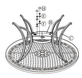
Step 4: After making any necessary adjustments to the alignment of the table legs and the leg connector bracket, use the hex bolt driver and hex wrench to tighten all nuts and bolts. Note: each bolt and nut must be tightened a few revolutions at a time. In order to apply equal pressure to all bolt joints, we recommend working in a cross corner (X fashion). Repeat until all bolts are tight. Do not over tighten. Over tightening may strip bolts. Cover all nuts and bolts with covers.
