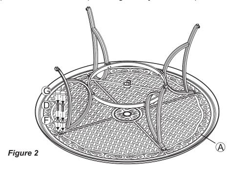
After making any necessary adjustments to the alignment of the table, use the hex bolt driver and hex wrench to tighten all bolts. Repeat until all bolts are tight. **Do not over tighten.** Over tightening may strip bolts. Cover all bolts with covers.
