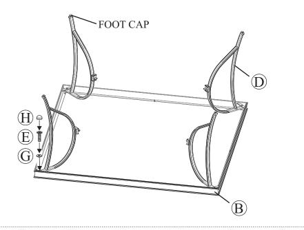
Attach a leg to the leg connector bracket by carefully guiding the bolts already in place on the table legs (each leg has two bolts) through the holes in the leg connector bracket. Add a washer and a nut to the end of each bolt as shown in **Fig.2**. **Hand tighten only 2-3 turns.** Repeat on the other three legs.
