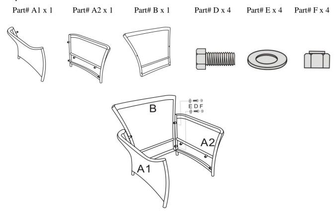
NOTE: DO NOT tighten the bolts completely at this step.
