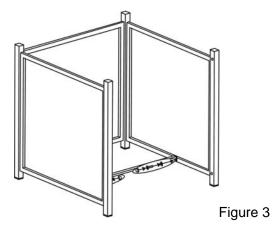
4. Attach the "L" connector to right side panel by using a 1/4"x15 mm bolt and washer as shown in Figure 4.Guide the bolt through the hole in the "L" connector, into the pre-drilled hole in the right side panel. **Do not over tighten.**
