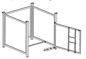
5. Put the door onto the bottom connector, guide the pin in the bottom connector into the hole on the underside of the door. Then guide the pin on the top connector into the hole in the topside of the door, use a 1/4"x15 mm bolt and washer to attach this top connector to the right side panel as shown in Figure 5. **Do not over tighten.**
