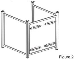
3. Attach the middle support to the side panels by using four 1/4"x15 mm bolts and washers as shown in Figure 3. Guide the bolts through the holes in the middle support, into the pre-drilled holes in the side panels. **Hand tighten only.**
