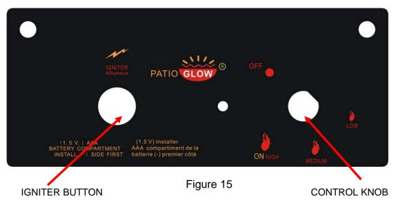
2. Push in the igniter button. You will hear a slight clicking sound. With the igniter button pushed in, push and turn the control knob to the "ON" position. the fire should light within a few seconds. Once the flame is lit, release the igniter button and continue to hold the control knob in for 10 to 15 seconds. Release the control knob. The control knob should pop back out and then remain lit.
