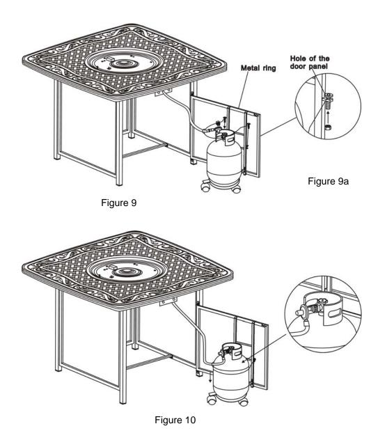
10. After making any necessary adjustments to the parts, use the hex bolt driver to tighten all bolts.
