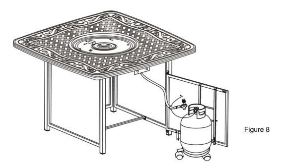
9. Attach the metal ring ( as shown in Figure 9) pre-fitted with gas hose which is connected to the table top , into the hole of the door panel, then use hex bolt driver to screw 1/4"x5mm nut , the gas tank has fixed as shown in Figure 9a. Connect the regulator as shown in Figure.10 Screw the black handle clock-wise to tighten. Turn the handle counter clock-wise to remove. The hose must point down. Check that the valve is turned all the way clockwise to the "OFF" position.
