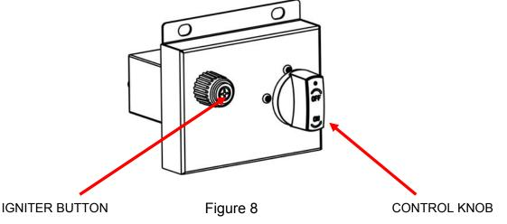
2. Push in the igniter button. You will hear a slight clicking sound. With the igniter button pushed in, push and turn the control knob to the "ON" position. The fire should light
