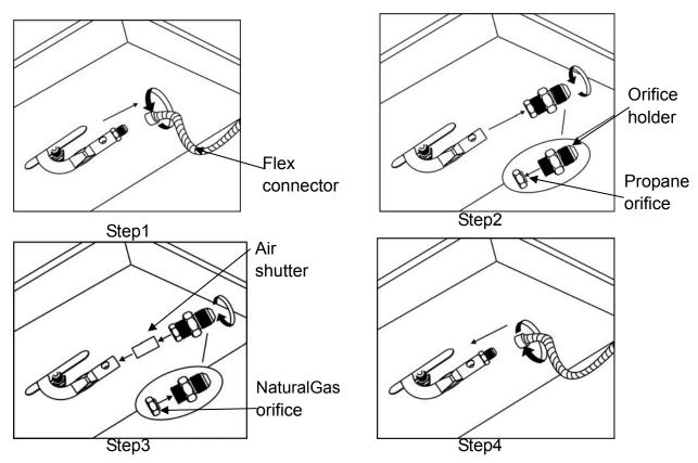
7. To convert the regulator from propane to natural gas, the appliance must be isolated from the gas supply piping system by closing its individual manual shot off valve. Ensure any pressure testing of the gas supply piping system is at test pressure equal to or less than 1/2 psi(3.5KPA)
