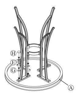
After making any necessary adjustments to the alignment of the table, use the hex bolt driver and hex wrench to tighten all bolts . **Note:** each bolt must be tightened a few revolutions at a time. In order to apply equal pressure to all bolt joints, we recommend working in a cross corner (X fashion). Repeat until all bolts are tight. **Do not over tighten.** Over tightening may strip bolts. Cover all bolts with covers.
