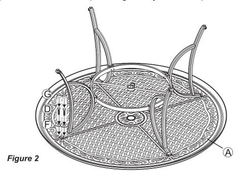
After making any necessary adjustments to the alignment of the table legs and the leg connector bracket, use the Open wrench to tighten all bolts.
