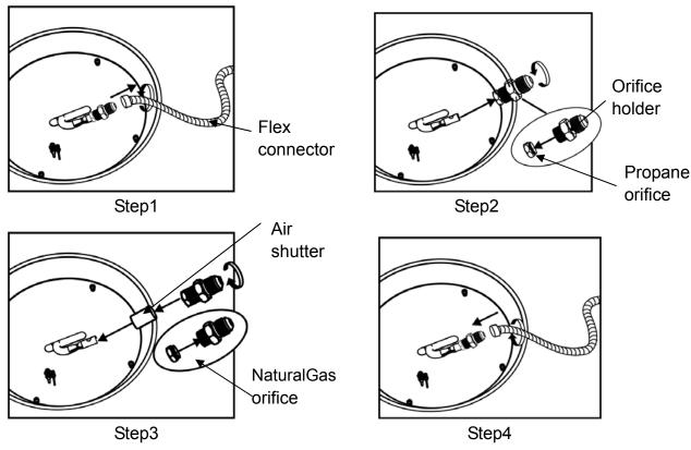
7. To convert the regulator from propane to natural gas the appliance must be isolated from the gas supply piping system by closing its individual manual shut off valve. Ensure any pressure testing of the gas supply piping system is at test pressure equal to or less than 1/2 psi(3.5KPA)
