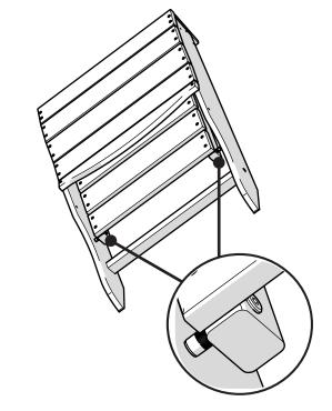
If the rivet nuts and bolts (included) are loose, hand-tighten them.
