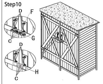
Secure 2x handles part F with 8x screw(D). Secure 2x part G with total 16x screw(C).
