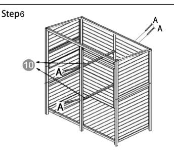
Put in 2x part<sup>1</sup>, secure with 4x screw(A) as shown.
