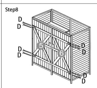
Attach doors part 3 and 6, secure hinges with 8x screw (D)
