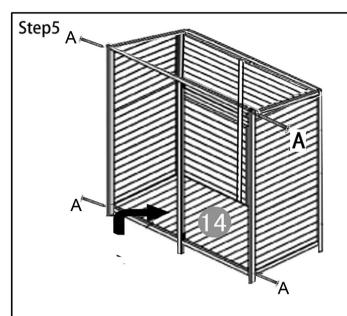
Connect the two parts finished in step 3 and 4, secure with 4x screw(A)
