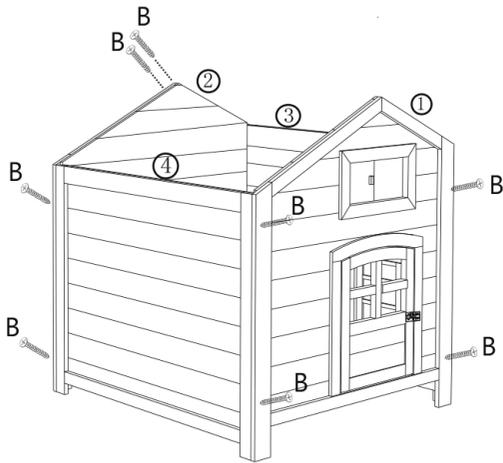
Secure part ①, ②, ③ and ④, by using 8x screw (B)
