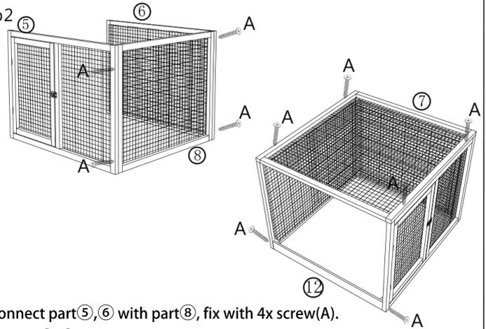
(1) Connect part ⑤, ⑥ with part ⑧, fix with 4x screw (A).
