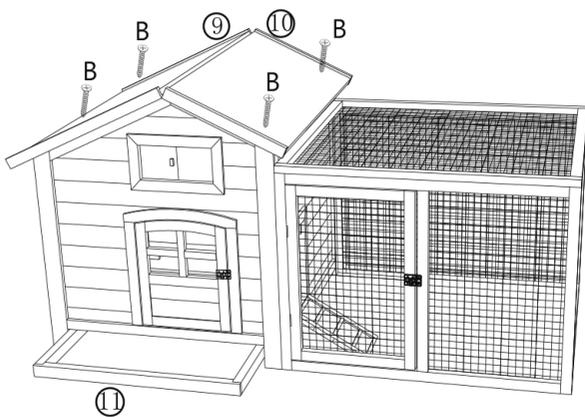
(1) Secure roof part ⑨ and ⑩, using 4x screw (B);
