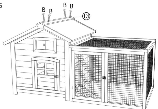
Attach roof cap part ⑬, secure with 4x screw (B).
