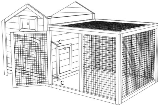
Connect the part finished in step 2 to main house. Open front door of part ⑤, secure with 2x screw (C).
