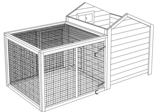
Turn to back, secure with 2x screw (C) as shown.
