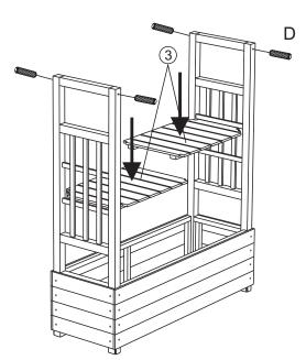
Place bottom part 3; Insert 4x dowels D as shown.
