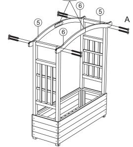
Use part (F) to connect part 5 and 6 as pictured, and fix them using 8x screw(C). Then fix them using total 8x screw(A).
