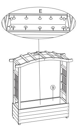
Place liner inside, and fix it using 14x pushpins (E). You may need a small hammer here.
