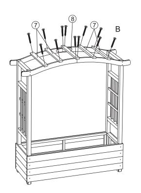
Fix part 8 using 4x screw(B) in the middle; Secure part 7 at roughly average distance, each using 2x screw(B).
