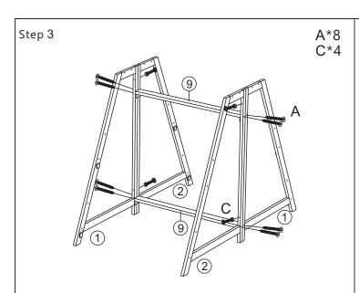
Secure part 1 with part 2 as shown, each side using 2x bolt & nut (C); Then secure 2x part 9 using 8x screw(A); layer, using 8x bolt & nut (C).
