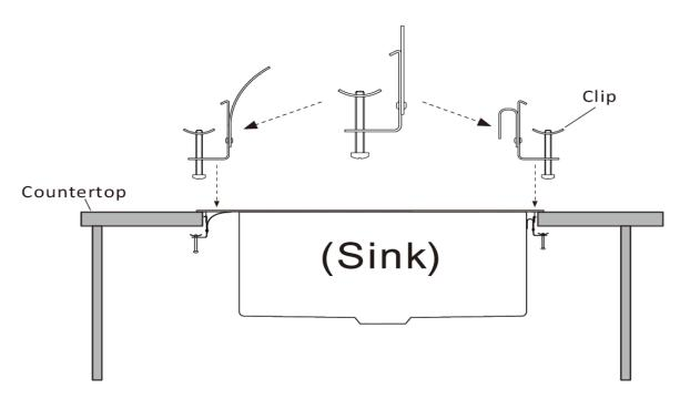
9. Once the sink in securely in place, use silicone caulk to seal any gaps where the sink meets the countertop.
