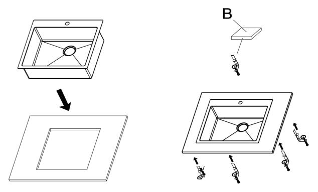
8. Tighten each screw until the sink is drawn down to the countertop.
