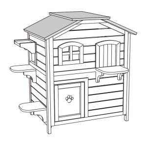
Roof part® is openable, and can be supported by the wood supporter inside front panel part①
