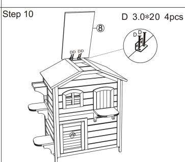
Put on roof part®, and secure hinges on the top surface of the back panel using 4x screw(D).
