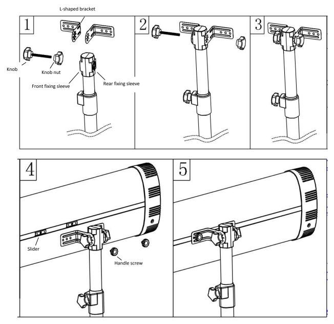
1) Parts that will be used for assembly are: tripod, knob screw, knob nut, L-shaped brackets.
