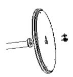
2. Tighten the adjustable feet onto the base.
