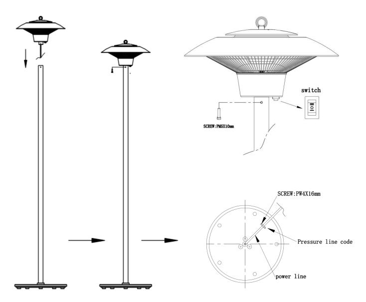
Note: This heater has two power settings that can be changed by the switch. Low heat operates at 750W and high heat operates at 1500W. This heater has a tip-over safety function. Once the heater is over a 45° angle, the heater will automatically turn OFF.
