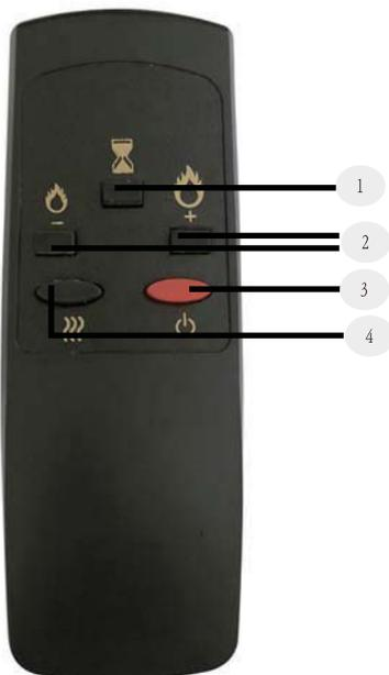
1. Heater Timer: Allows you to leave your heater on with an automatic timer for shut off. You can set your heater to be on for 1/2 hour increments starting at a 1/2 hour up to a maximum of 7-1/2 hours – press once for each 1/2 hour increment. After you reach 7-1/2 hours the next press will shut off the feature.
