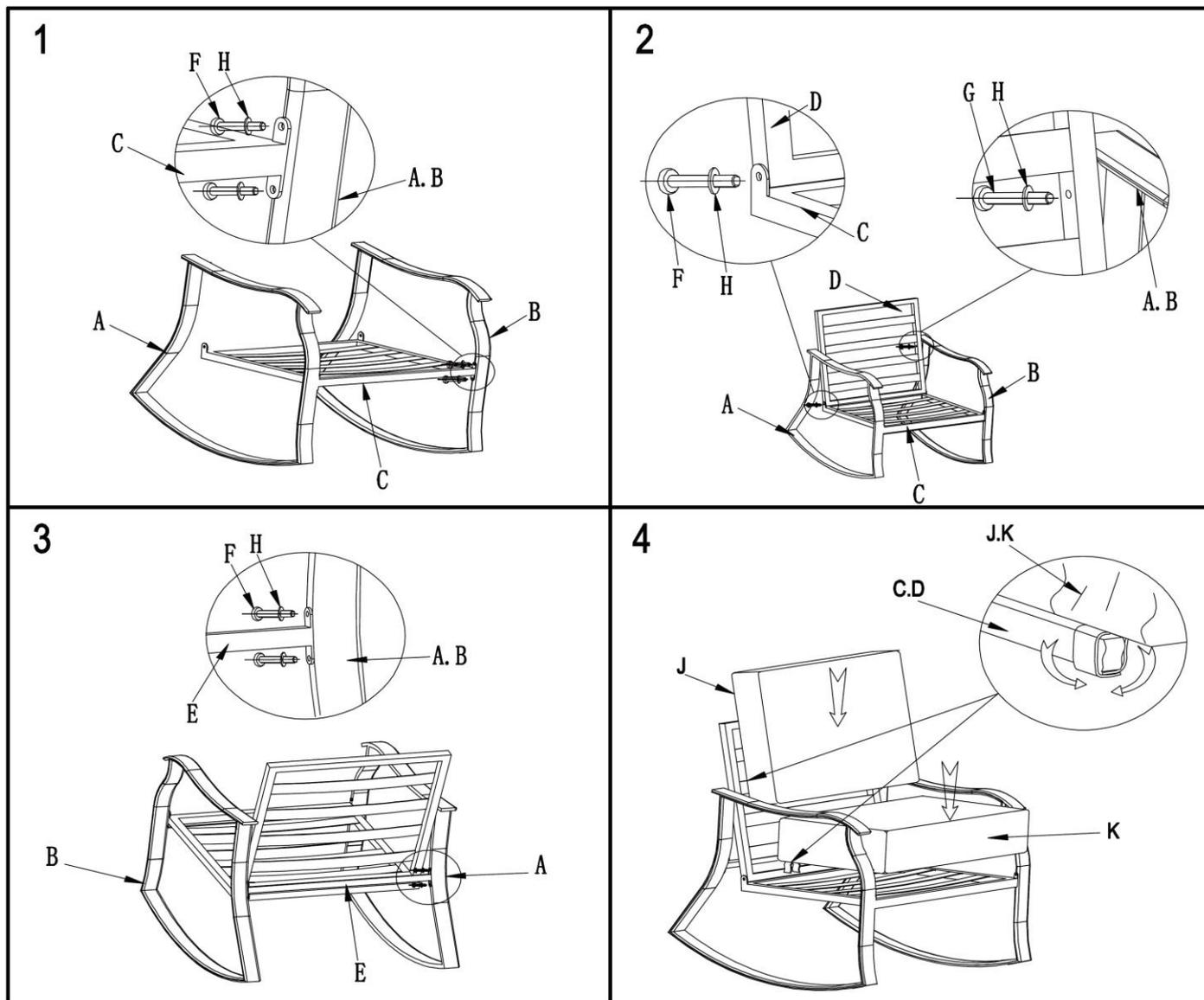
Tighten all the bolts using Allen Key (I). Repeat the steps for second chair.
