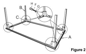
Step 4. Check the alignment and adjust if necessary. Once the alignment is correct, tighten all bolts with open wrench ( I). Cover all bolts with bolt caps(H).
