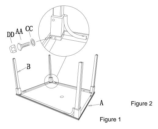
Step 3. Loosely attach the support tube (C) to the table leg (B) and table top (A) with bolts (BB) and washer (CC) as shown in figure 2.
