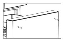
1. Before the refrigerator door handle is installed (note: the anchor bolts of the handle are in the accessory bag, and all steps should be performed at the right and left two mounting positions simultaneously.
