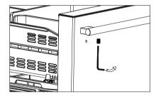
4. Wait until the handle fits perfectly with the door body, and then use a hexagonal wrench to tighten the locking screw inside the handle part.
