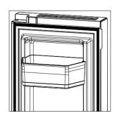
1. Place the tray above the mounting position and force the door up to the bottom, completing the installation when it cannot continue to move down.
