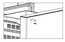
2. Screw the locating bolt into the bolt hole of the door body and secure it.
