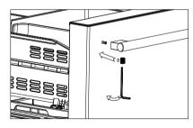
3. Loosen the locking screw inside the handle part with a hexagonal wrench first, then align the handle with the positioning bolt and insert it into the positioning bolt (note: the handle locking screw is installed facing down).
