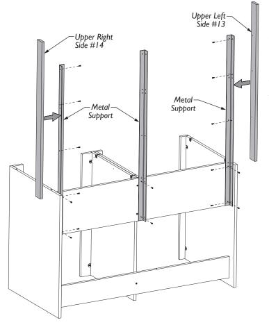
Attach (3) Metal Supports to the back of the Upper Brace and the Left and Right Side Panels using (10) 5/8" Pan Head Screws.
