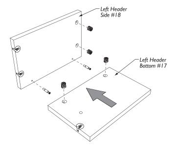
Insert (2) Mini-Fix Cams into the slots in Left Header Bottom #17. Insert (2) Mini-Fix Cams into the slots in Left Header Side #18. Screw (2) Mini-Fix Posts into Left Header Side #18.
