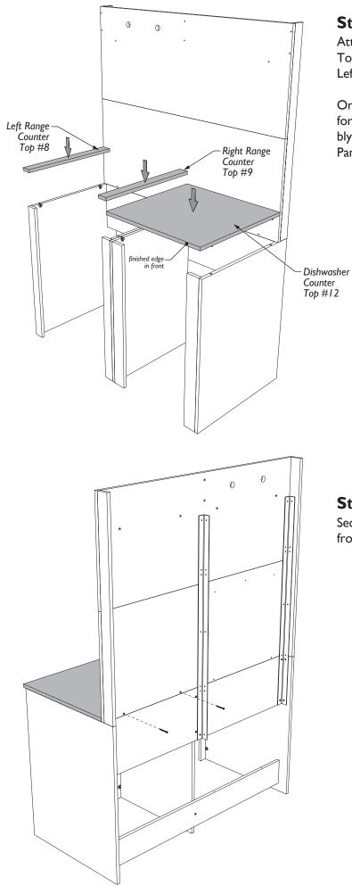
Attach Left Range Counter Top #8 and Right Range Counter Top #9 to the assembly and tighten the Rafix Cams in the Left Side Panel and Divider Panel Cleat.
