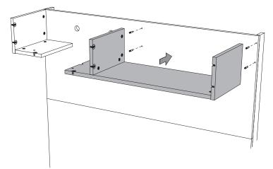
Screw (4) Mini-Fix Screw Posts into the Upper Back. Attach the Right Header assembly to the Back Panel. Use a screwdriver to turn the Mini-fix Cam's one quarter turn to secure it in place.
