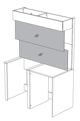
Tape the (2) Backsplash Graphics to the Back Panels. Each one is labeled on the back side to identify the top edge.
