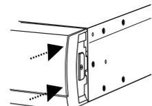
5. Gradually apply pressure to the left and right ends of the front panel until you hear the latches 'click'.
