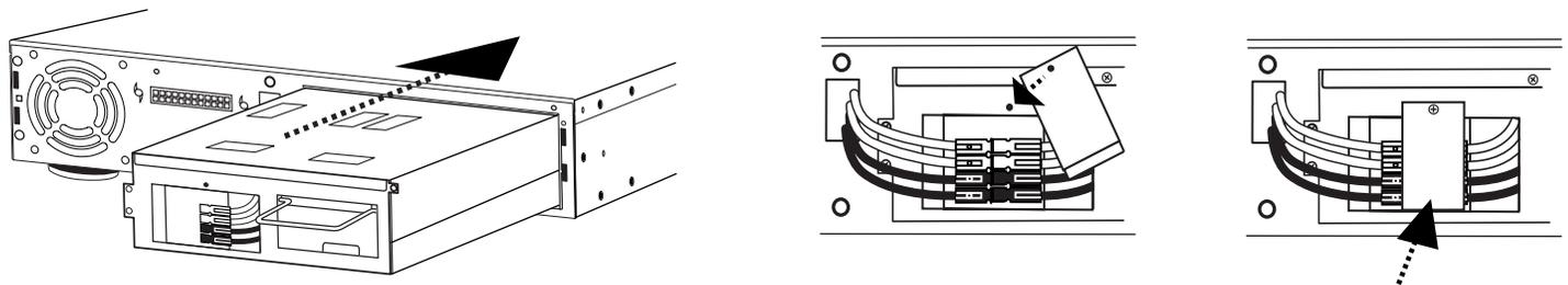
5. Install the new battery pack into the unit. **DO NOT ATTEMPT TO REPLACE THE BATTERIES IN THE ORIGINAL BATTERY PACK. IMPROPER INSTALLATION CAN RESULT IN FIRE OR BATTERY LEAKAGE.**
