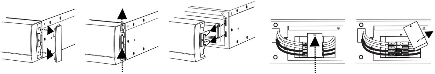
1. Remove the front panel. Remove the rubber end caps and pull up on the latch mechanism. Once the latch mechanism stops,
