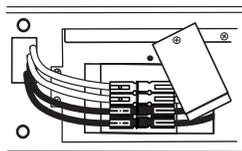
2. Verify that the battery connectors are connected, red-to-red, black-to-black. If not connected, perform steps 2 and 6 in the BATTERY REPLACEMENT section.
