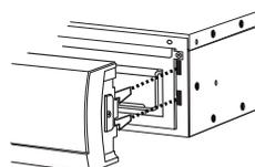
4. Carefully align the front panel connector and latches with the F1500-UPS.
