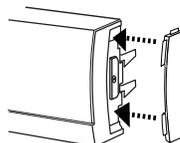
3. (Optional) Install the supplied rubber end-caps to the sides of the front panel. Push the curved edge of the end-cap into the mating slots of the front panel.
