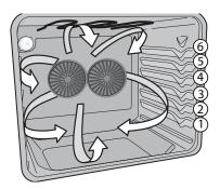
Figure 17: Convection air flow
