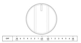
Figure 4: Dual element control for 9 or 12 inch burner To operate the dual surface element:
