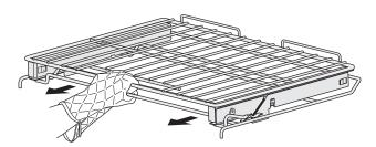
Figure 10: Pull rack to stop position
