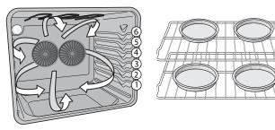
Figure 15: Rack positions Figure 16: Pan spacing
