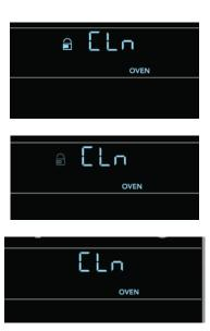
Figure 38: Clean lock icon blinks as door unlocks
