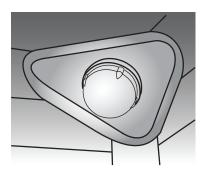
Figure 46: Oven light protected by glass shield
