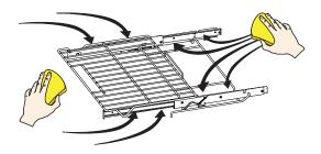
Shake graphite lubrication very well before applying. Apply to loading guides, and rotation pin. Repeat on both sides of the glide rack.
