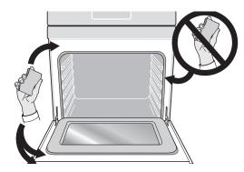
Figure 30: Clean around the oven door gasket
