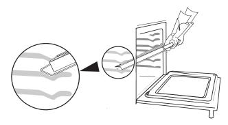
Figure 11: Remove and replace using both hands
