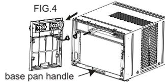
7. Remove shipping screws from top of unit and also on both sides by the base if installed. (See FIG.5)
