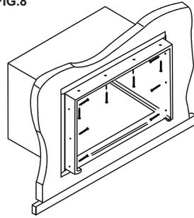
6. Install air conditioner into cabinet by following all steps in Step 9 of Window Mounting.
