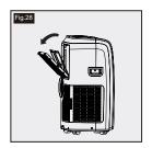
To keep your appliance working efficiently, you should clean the filter every week of operation. The evaporator filter can take out like Fig. 28. The condenser filters are two pieces.
