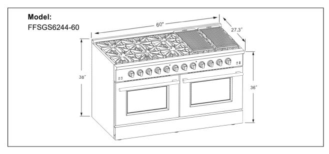
This range may be installed directly adjacent to existing countertop-height cabinets (36" or 91.5 cm from the floor). To achieve the best look, the cooktop should be level with the cabinet countertop. This can be accomplished by raising the unit using the adjustment spindles on the legs.
