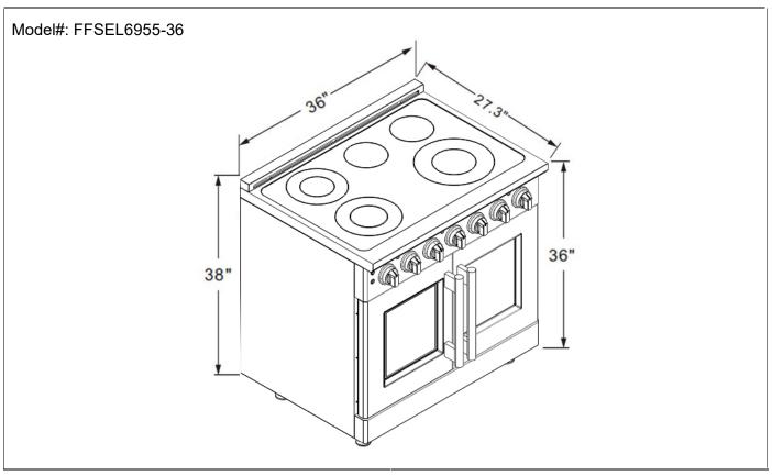
This range may be installed directly adjacent to existing countertop-height cabinets (36" or 91.5 cm from the floor). To achieve the best look, the cooktop should be level with the cabinet countertop. This can be accomplished by raising the unit using the adjustment spindles on the legs.
