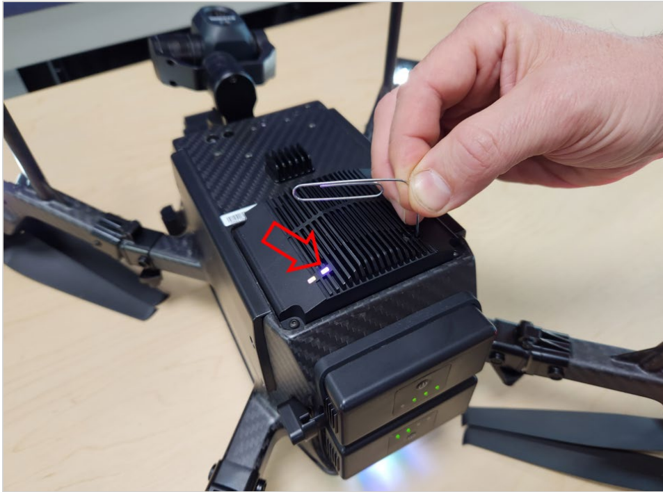
FIGURE 7.L PRESSING THE PAIR BUTTON (PAIRING LIGHT FLASHING)
