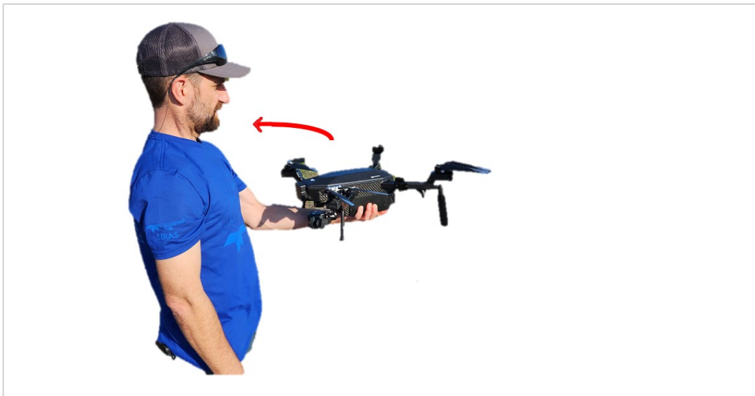
FIGURE 8.B COMPASS CALIBRATION STEP 2: HORIZONTAL ROTATION, LEVEL
