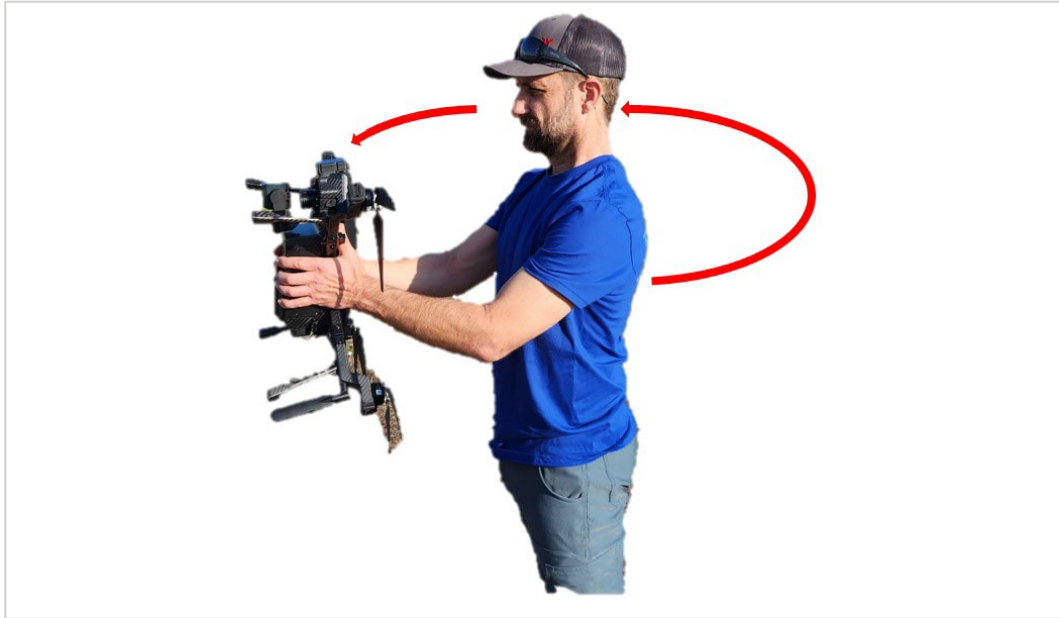
FIGURE 8.D COMPASS CALIBRATION STEP 3: HORIZONTAL ROTATION, NOSE-UP
