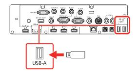
**Note:** Connect the flash drive directly to the projector. Do not use a hub or your settings may not be saved correctly.
