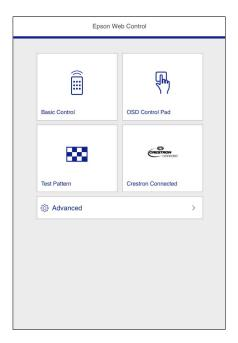
4. To control projection remotely, select the **Basic Control** option from the Web Control screen.
