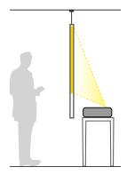
Wherever you set up the projector, make sure to position it squarely in front of the screen, not at an angle.
