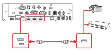
**Note:** If you have problems hearing audio through the HDMI connection, you can use one of the projector's audio ports instead to play sound. Connect one end of an optional 3.5 mm stereo mini-jack audio cable to one of the projector's audio ports and the other end to your computer's audio out port. Then select the audio port you connected to as the **HDMI Audio Output** setting in the Signal I/O menu.
