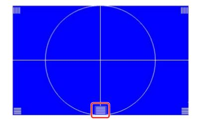
7. Once the center reference point is in focus, check that the corner reference points are also in focus.
