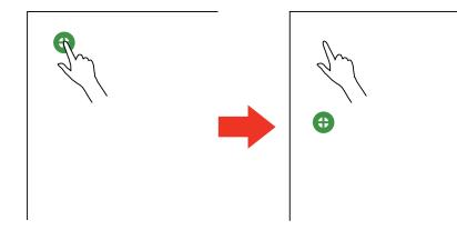
**Note:** For the most accurate calibration, make sure you touch the center of the circle with the tip of your finger.
