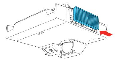
8. Close the air filter cover and tighten the screws.
