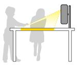
Mounted on the wall or ceiling and projecting from behind a translucent screen (interactive features not supported)
