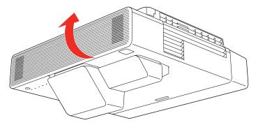
6. Move the focus lever and adjust the focus using the center reference point of the projected screen.
