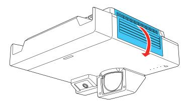
4. Pull the air filter out of the projector.
