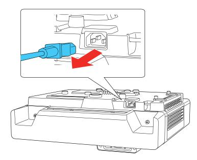
**Caution:** To avoid damaging the projector or laser, never unplug the power cord when the Status light is on or flashing.
