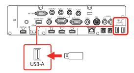
**Note:** Connect the flash drive directly to the projector. Do not use a hub or your settings may not be saved correctly.
