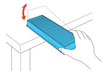
**Caution:** Do not use excessive force when tapping the air filter, or it may crack and become unusable. Do not rinse the air filter in water, or use any detergent or solvent to clean it. Do not use canned air; the gases may leave a flammable residue, or push dust and debris into the projector's optics or other sensitive areas.
