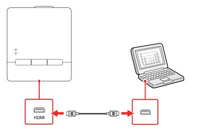
3. Press the **1** or **2** button on the control pad to select the port your computer is connected to.
