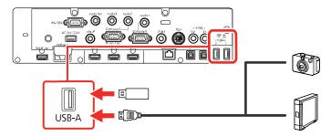
**Note:** Use the USB cable supplied with or specified for use with your device. Do not connect a USB hub or a USB cable longer than 10 feet (3 m), or the device may not operate correctly.
