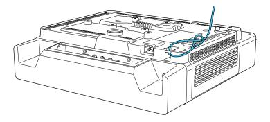
**Note:** Do not pass drop-prevention cables through the security cable attachment point when mounting the projector on a wall or ceiling.
