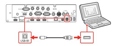
**Note:** If you use a USB hub, the connection may not operate properly. Connect the USB cable directly to the projector.
