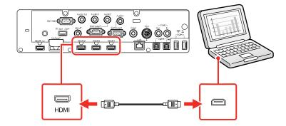
**Note:** If you have problems hearing audio through the HDMI connection, connect one end of an optional 3.5 mm stereo mini-jack audio cable to the projector's **Audio** port and the other end to your computer's audio out port. Then select the audio port you connected to as the **HDMI Audio Output** setting in the Signal I/O menu.
