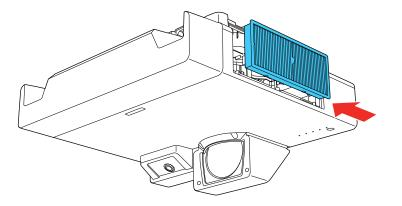
6. Close the air filter cover and tighten the screws.
