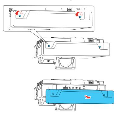
To attach the cable cover, replace the cable cover and tighten the cable cover screws.
