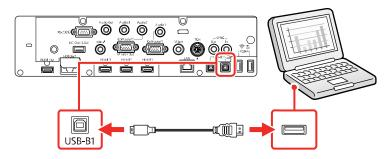
**Note:** If your computer is connected to the projector's **HDMI3** port, connect the USB cable to the projector's **USB-B2** port. You can change the HDMI port associated with the USB-B2 port by changing the **USB-B2** setting in the projector's **Pen/Touch** > **PC Interactivity** menu.
