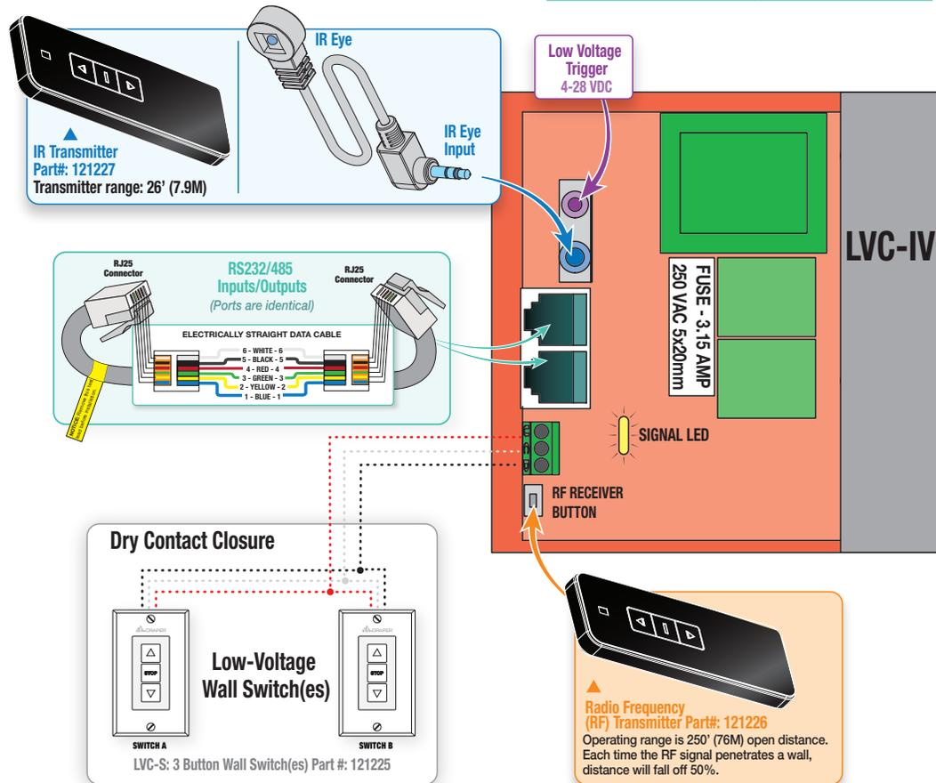
The 120V LVC-IV also used as a Single-Pole, Double-Throw dry closure to control equipment by the same means listed above.
