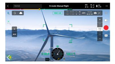
Zoom Frame: after switching to the wide mode as the main view, the field of view and camera zoom ratio will be displayed on the zoom frame.
