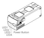
The battery level LEDs display the power level of the battery during charging and discharging. The statuses of the LEDs are defined below:
