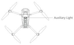
▲ The auxiliary light will automatically turn on in low-light environments when the flight altitude is under 5 m. Note that the positioning performance of the vision systems may be affected. Fly with caution if the GNSS signal is weak.
