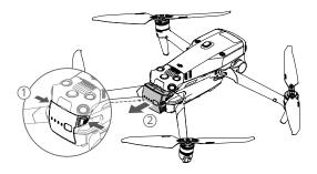
$\wedge$  • DO NOT insert or remove the battery while the aircraft is powered on.
