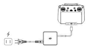
:ඊ는 Fully discharge and charge the remote controller every three months. The battery depletes when stored for an extended period.
