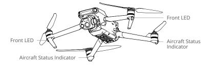
When the aircraft is powered on, but the motors are not running, the front LEDs glow solid red to display the orientation of the aircraft.
