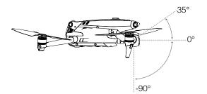
Use the gimbal dial on the remote controller to control the tilt of the camera. Alternatively, enter the camera view in DJI Pilot 2. Press the screen until a circle appears and drag the circle up and down to control the tilt of the camera.
