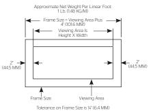
Tolerance on Frame Size is 1/4" (6.4 MM)
