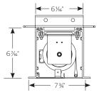
3/8" Threaded Rod (Not Included) Attached to Mounting Bracket
