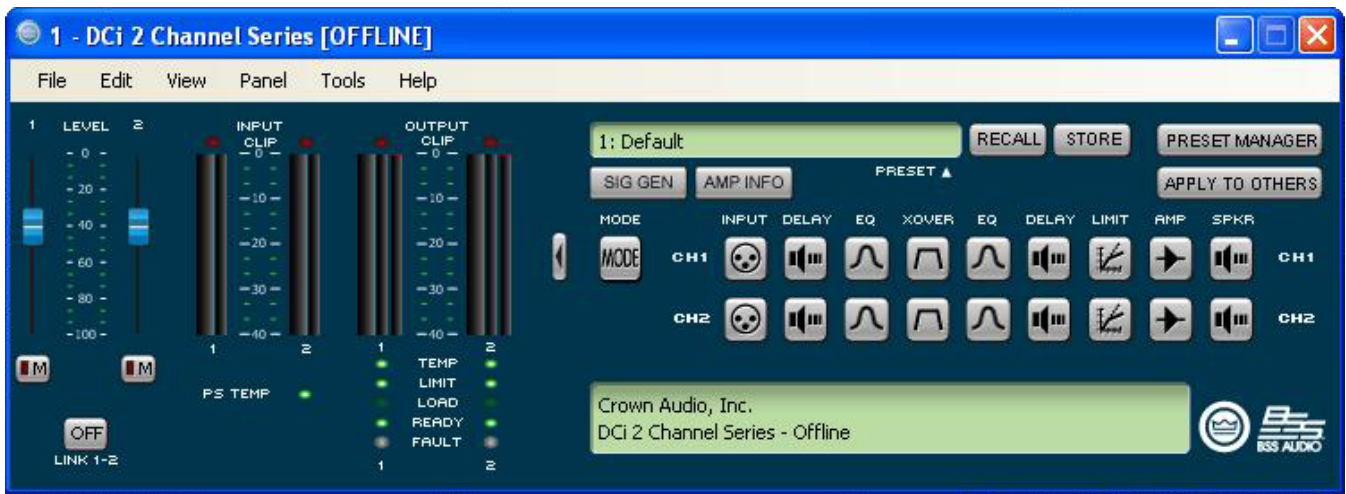
Figure 13 (above) shows the DriveCore Install 2 channel configuration page. The 4 and 8 channel amplifier configuration pages have the same feature set. The DriveCore Install Network amplifier includes Digital Signal Processing (DSP), multiple input/output routing options and a comprehensive diagnostics feature set. All of these features can be adjusted in from the configuration page.
