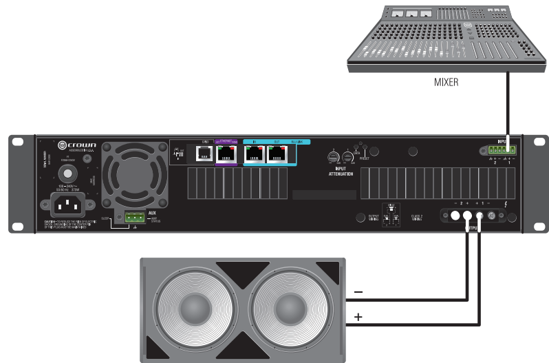
Figure 21 System Wiring Bridge Mode
