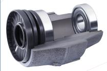
Two commercial grade SKF bearings are sealed for maximum protection. Three individual seals with 5 lips provide a water-tight barrier around the drive shaft to protect the bearings from damaging moisture.
