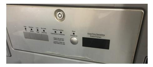
8. Remove the front control panel frame by removing the four screws shown.
