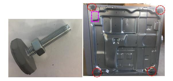
10. Remove the four adjustable feet from the dryer and remove the rectangular "knockout" plate as indicated in the picture. Loosen slightly, but do not remove, the 4 shouldered self-extrusion screws which are already attached under the base panel of the DLHS dryer.
