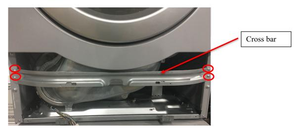
14. Feed the hex head screw previously removed in step #8 through the base of the upper machine and feed back into the threaded hole in FRONT-RIGHT mounting bracket of the lower machine using a socket ratchet, locking the position of the two machines relative to each. WARNING: This step must be done correctly to prevent the upper machine from being pushed backwards. Note: for COIN metered machines see step 16.
