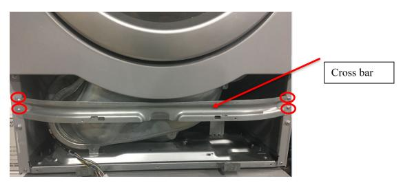
10. Feed the hex head screw removed in step #2 through the base of the upper machine and feed back into the threaded hole in the FRONT-RIGHT mounting bracket of the lower machine using a socket ratchet, locking the position of the two machines relative to each. WARNING: This step must be done correctly to prevent the upper machine from being pushed backwards. Note: for COIN metered machines see step 11.
