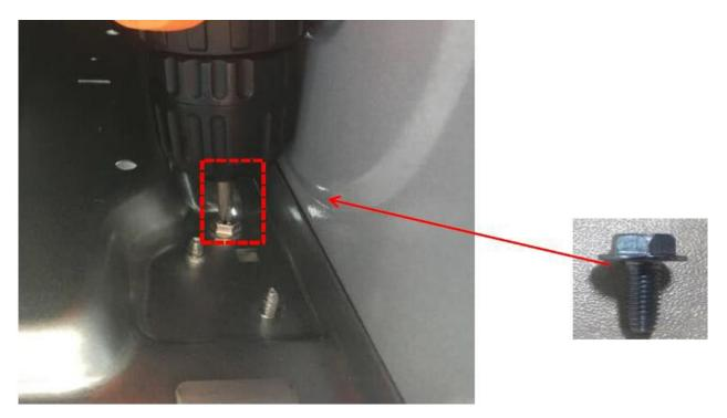
11. Reattach cross bar and panel frame but do not remount the control panel.
