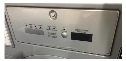
2. Remove the front control panel frame by removing the four screws shown.
