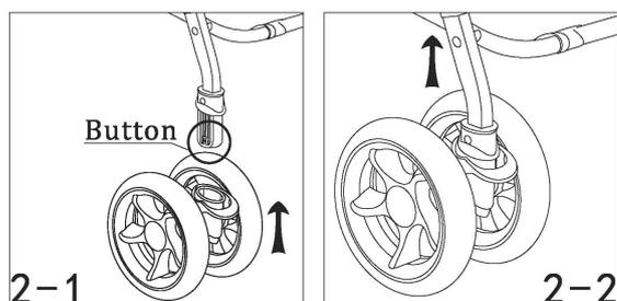
5. Assemble front wheels: Insert each wheel onto the respective leg and push upward until you hear a "click".
