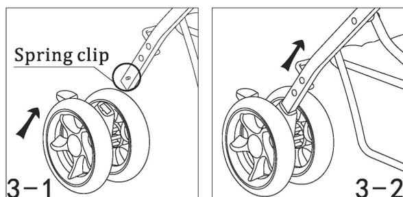
7. To assemble rear wheels: Hold the rear wheels with the red brake in the back, and insert the rear wheels onto the rear leg until the spring clip goes into the slot of the wheels connector.
