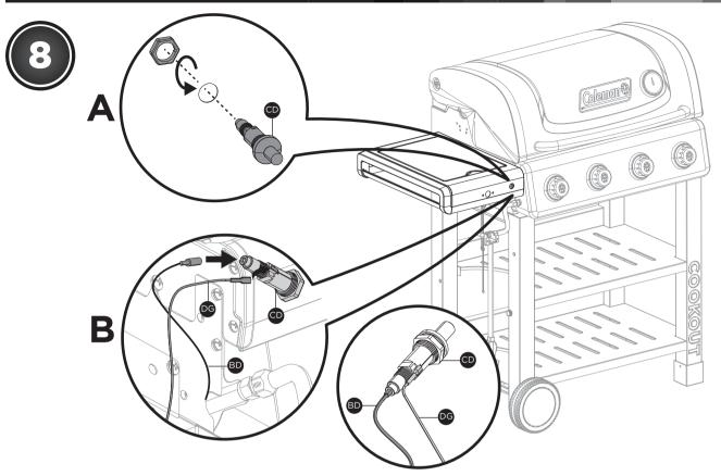
**ATTENTION:** Figure B illustrates how to connect the electrode set, main burner (BD) and the side burner electrode wire (DG) to the ignitor (CD). Locate both wires on the left side of the burner box. The side burner electrode wire (DG) has a black connector which connects to the ignitor (CD) and a red connector which will be assembled in step 11.
